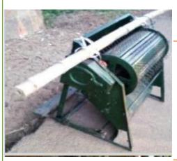
**Pedal powered** INR 3000-6000 Foot is used to pedal and turn the drum Threshing capacity: 50-60 kg/hr
